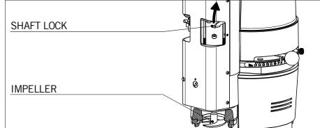
The impeller must be cleaned only by skilled technical personnel, **after disconnecting the appliance from the power supply**, according to the following instructions:
