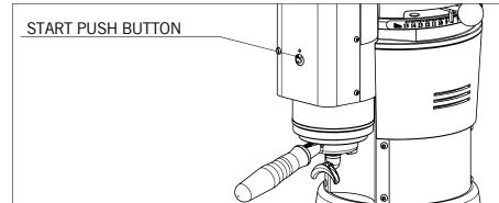
In order to power up the appliance, turn the on-off switch knob to I. Engage the filter holder directly to the appliance (**apply only a light amount of torque; if the grinder shifts on the counter top, you are using too much force**).
