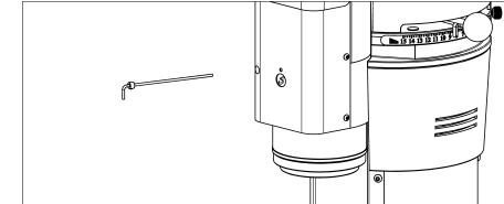
The cleaning of the coffee outlet chute must be made by the insertion of the tool 5.372.5 into the hole (caution when moving the tool).
