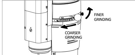
In order to achieve finer or coarser grinding, move the grinding adjustment level. To increase the coarseness of the ground coffee, the adjustment level must be rotated clockwise; to increase the fineness, turn the level anticlockwise.
