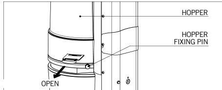
Make sure the hopper is positioned correctly on the appliance and fixed to the casing with relevant pins.
