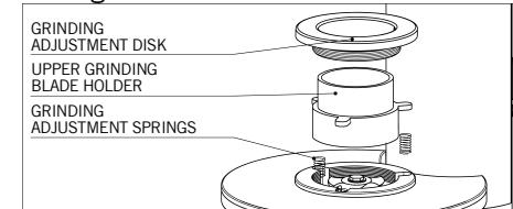
Please check that the grinding adjustment springs are on their place. Having refitted the upper grinding blade holder in the relevant slot, please lubricate, with grease suitable for food contact, the threads of the grinding adjustment disk and its underneath surface which touches the upper grinding blade holder. Screw the adjustment disk by turning it anticlockwise, place the adjustment level and fix it on adjustment disk with the relevant screws
