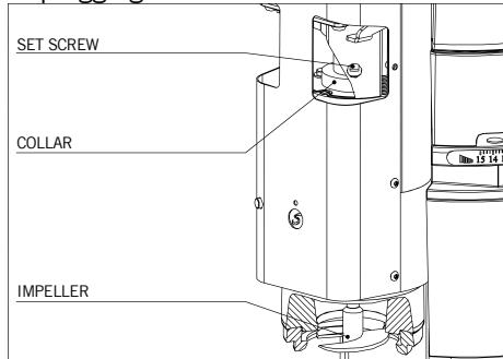
It is possible to change the dosage quantity by raising or lowering the height of the impeller.
