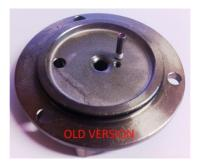
This cap has been now redesigned, so that the ruby gigleur is placed between the flowmeter outlet and the solenoid valve inlet (SEE IMAGES BELOW). In addition the inlet of the flowmeter has been further restricted from 1,1mm to 0,9mm. This change is affecting ALL GB5&FB80 from machine s/n 5679 (AV) and s/n 5680 (EE).
