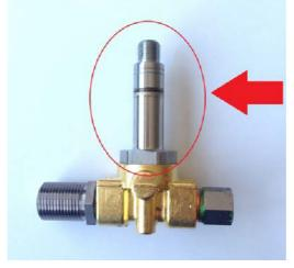
To help mitigate the issue, La Marzocco has improved the material of the two-way solenoid plunger sleeve from 303 series stainless steel to 316L series stainless steel. This improvement was introduced to machines manufactured in March 2015 starting with serial number Strada 1936, Linea PB 1767, GS3 5048, GB5 012944, Linea Classic 044938.
