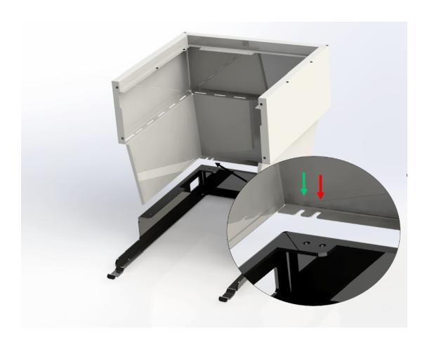
In order to add clearance around the pump motor, the screw position has been moved. Both the frame and the panel have 2 positions for holding the screw. This is in order to guarantee the interchangeability with previous frames or panels.
