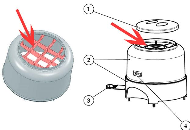
The shape of the inlet hole has been modified to facilitate easier loading of coffee. The new grid (shown on left) is positioned a step below the rim unlike the previous design (shown on right) and includes the same geometry as that of the Vulcano Swift hopper.
